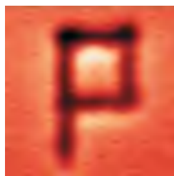
Figure 13. Magnetic lithography. Letter "P" is written by magnetic tip in continuous CoPt film with perpendicular anisotropy by similar way as shown in Figure 12.
